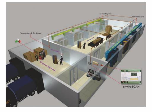
enviroSCAN, the Multi Channel Scanners & Data Loggers and the Web based Enviro Multiple Warehouses Monitoring Software, together monitor the temperature and RH under which your vital medicines and vaccines are stored in the network of your warehouses in the Cool Chain and thus assist you in **your Good Distribution Practices (GDP)**
