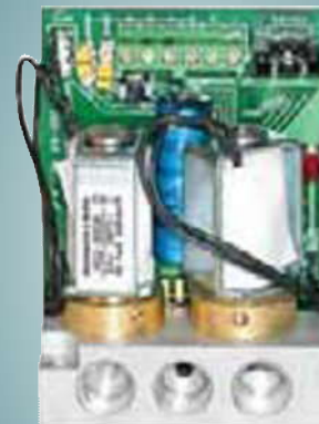
Type 341 I Digital Circuit-Card Pressure Regulators
