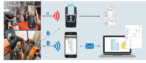
The testo 330-1/-2 LX transfers measurement results by infrared to the Testo IR printer, which you can use to print out the measurement report.
