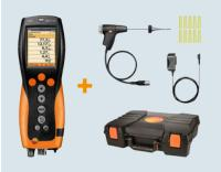
Set consists of • Flue gas analyzer testo 300-1 LX with O<sub>2</sub> sensor, CO sensor and Bluetooth® • International mains unit • Basic flue gas probe, length 180 mm, Ø 6 mm • Spare dirt filter (10 off) • System case for instrument, probes and accessories
