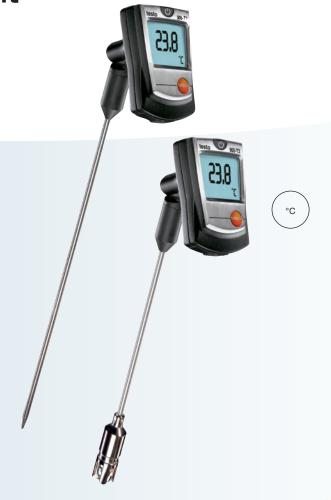
The testo 905-T1 is a particularly fast penetration thermometer with a broad measuring range of -50 to +350 °C, in the short term even up to +500 °C (1 to 2 minutes). The measuring instrument has a professional industrial sensor (thermocouple Type K). It has an excellent level of accuracy, especially in the upper measuring range. The testo 905-T2 is a surface thermometer with a broad measuring range of -50 to+350 °C, in the short term
