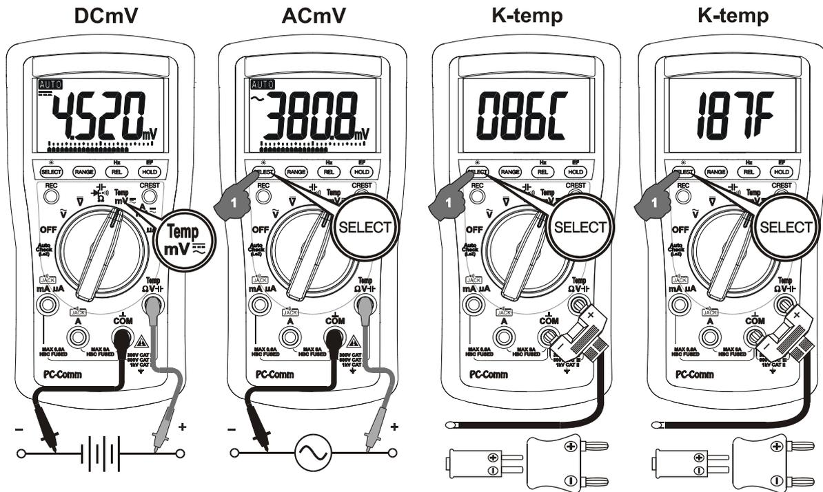
Note: Be sure to insert the banana plug K-type temperature bead probe AMD 9023 with correct  $+$   $-$  polarities. You can also use a plug adapter AMD 9024 (Optional purchase) with banana pins to K-type socket to adapt other standard K type mini plug temperature probes.
