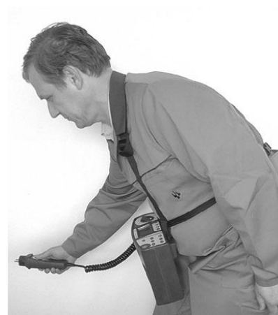
The instrument is hung around operator's neck and fixed to his body with back belt - stable position.
