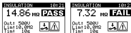
Examples of insulation resistance measurement results
