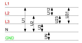
Figure 5.1: Phase and phase-to-phase (line) voltage
