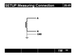
Figure 4.6: Choosing 1-phase 3-wire system on instrument
