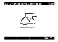
Figure 4.4: Choosing 3-phase 3-wire system on instrument
