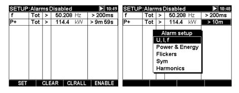
Figure 3.42: Alarms setup screen.
