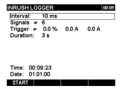
Figure 3.24: Inrush logger setup screens.
