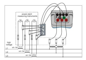
Figure 4.9: Connecting instrument to the existing current transformers in medium voltage system
