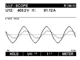
Figure 3.7: Voltage and current waveform (single mode)
