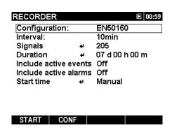
Figure 3.34: Basic recorder setup screen
