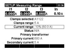
Figure 4.12: Selecting 10% of current clamps
