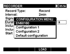
Figure 5.12: Predefined EN50160 recorder configuration
