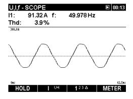
Figure 3.6: Current waveform
