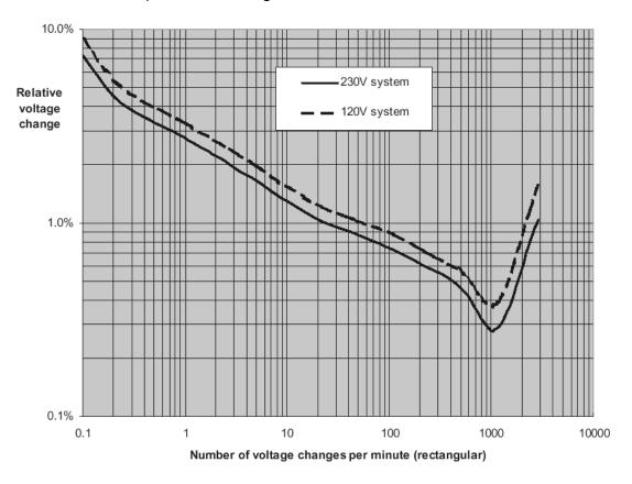
Figure 5.7: Curve of equal severity (Pst=1) for rectangular voltage changes on LV power supply systems
