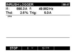
Figure 3.25: Inrush logger capture screen.
