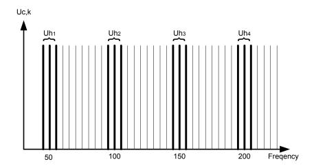
Figure 5.5: Illustration of harmonic subgroup for 50 Hz supply
