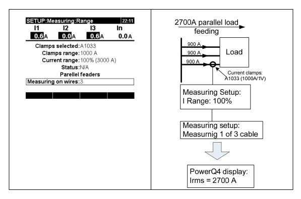
Figure 4.10: Parallel feeding of large load
