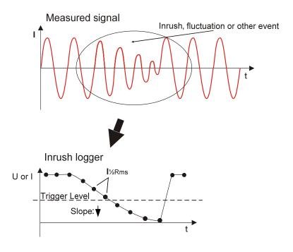
Figure 5.10: Inrush (waveform and RMS)
