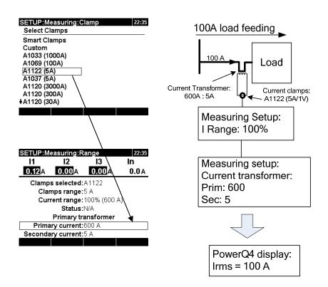
Figure 4.11: Current clamps selection for indirect current measurement
