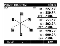
Figure 3.32: Phase diagram screen.
