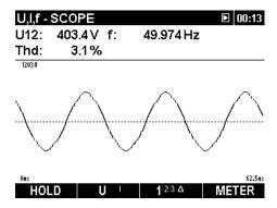
Figure 3.5: Voltage waveform
