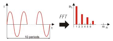
Figure 5.4: Current and voltage harmonics
