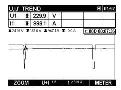
Figure 3.10: Voltage and current trend (single mode)
