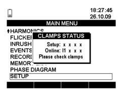
Figure 4.14: Automatically recognized clamps setup
