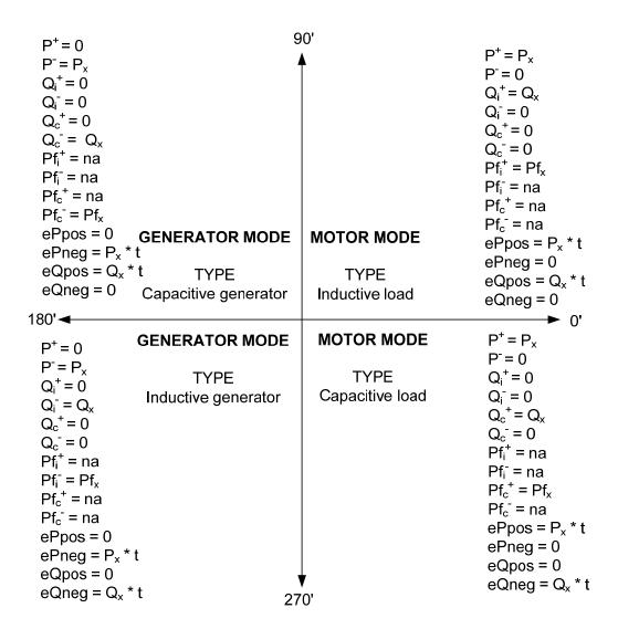
Figure 1: Motor/generator and inductive/capacitive phase/polarity diagram
