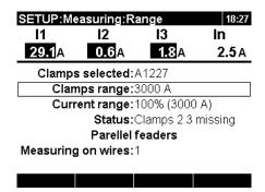
Figure 4.13: Automatically recognised clamps setup
