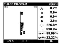
Figure 3.33: Symmetry diagram screen
