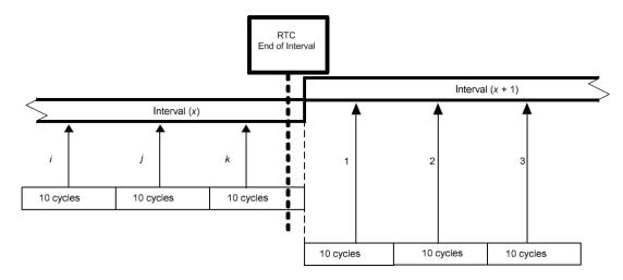
Figure 5.9: Synchronization and aggregation of 10 cycle intervals
