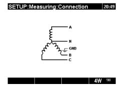
Figure 4.2: Choosing 3-phase 4-wire system on instrument
