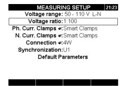
Figure 4.8: Voltage ratio for 11kV/110kV transformer example
