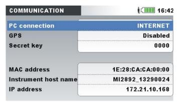
Figure 4.24: Internet connection setup screen
