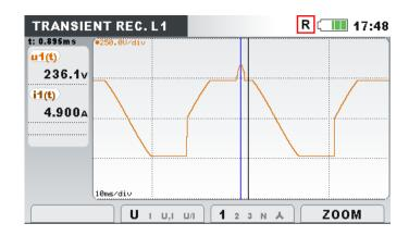
Figure 3.53: Captured transient recorder screen
