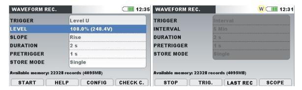
Figure 3.48: Waveform recorder setup screen
