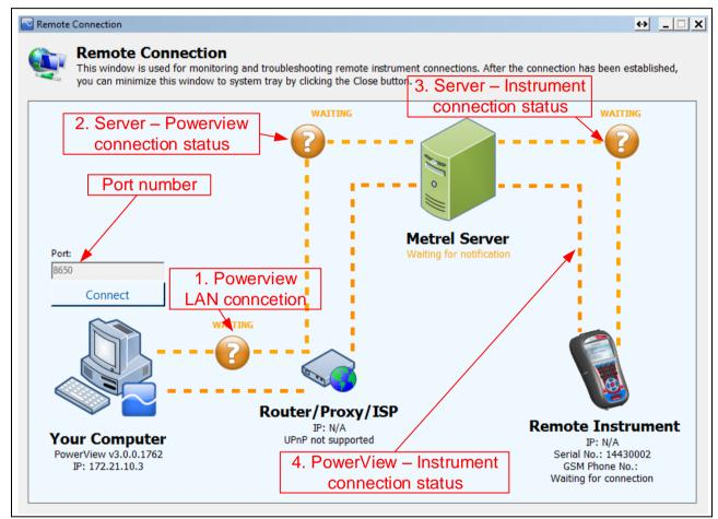
Figure 4.26: PowerView v3.0 remote connection monitor
