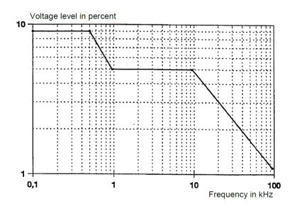
Figure 5.26: Mains signalling voltage level limits according to EN50160
