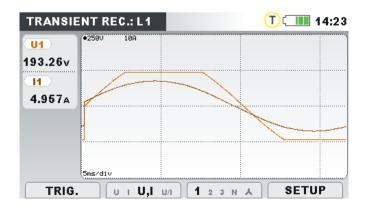
Figure 3.52: Transient recorder capture screen
