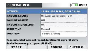
Figure 5.27: Predefined EN50160 recorder configuration
