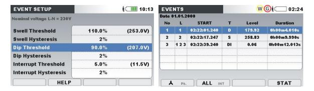
Figure 5.11: Voltage dip related screens on the instrument
