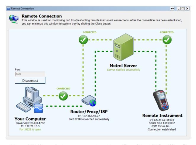
Figure 4.29: Remote instrument connection to PowerView v3.0 established (Step 4)
