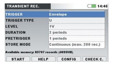
Figure 3.51: Transient recorder setup screen
