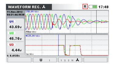
Figure 3.50: Captured waveform recorder screen
