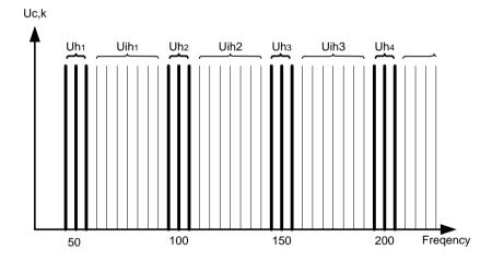
Figure 5.7: Illustration of harmonics / interharmonics subgroup for 50 Hz supply
