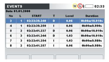
Figure 3.55: Voltage event in detail view screen
