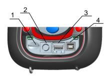
Figure 2.3: Side connector panel
