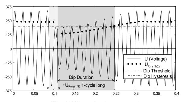
Figure 5.9:U<sub>Rms(1/2)</sub> 1-cycle measurement
