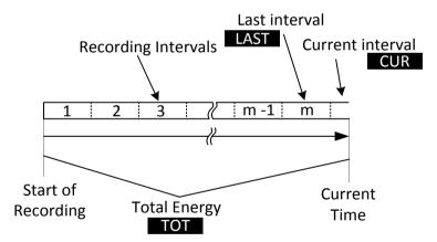
Figure 5.5: Instrument energy counters
