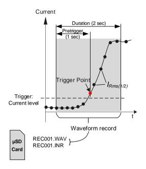
Figure 5.20: Current Level Triggering (Inrush)
