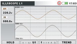
Figure 3.15: Voltage and current waveform (dual mode)
