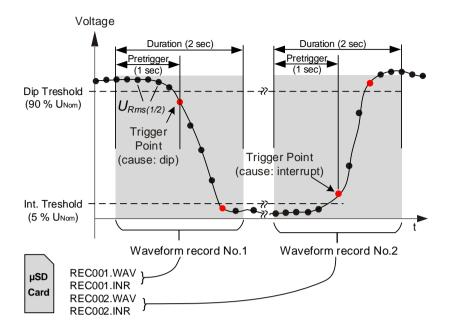
Figure 5.18: Voltage Event Triggering
