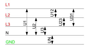
Figure 5.1: Phase and Phase-to-phase (line) voltage
