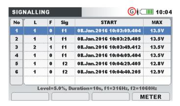
Figure 3.45: Signalling table screen
