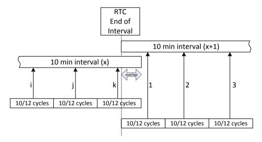
Figure 5.14: Synchronization and aggregation of 10/12 cycle intervals
