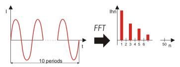
Figure 5.6: Current and voltage harmonics
