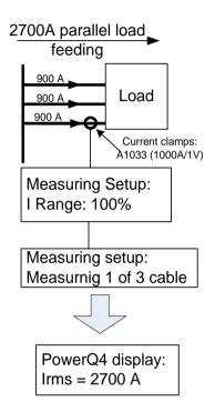
Figure 4.15: Parallel feeding of large load
