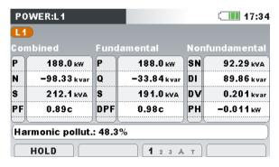
Figure 3.24: Detailed power measurements at phase L1
