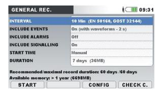
Figure 3.46: General recorder setup screen
