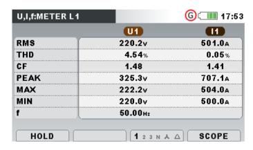
Figure 3.10: U, I, f meter phase table screens (L1, L2, L3, N)
