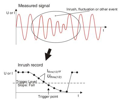
Figure 5.22: Level triggering
