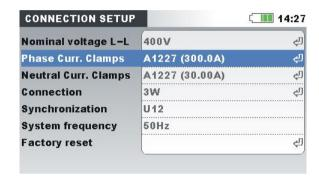
Figure 4.18: Automatically recognised clamps setup
