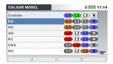
Figure 3.77: Colour representation of phase voltages
