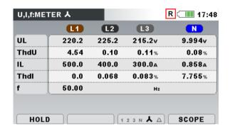
Figure 3.63: U,I,f meter screen in recalled snapshot record
