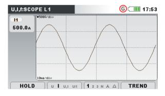
Figure 3.13: Current only waveform
