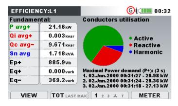
Figure 3.29: Energy efficiency screen
