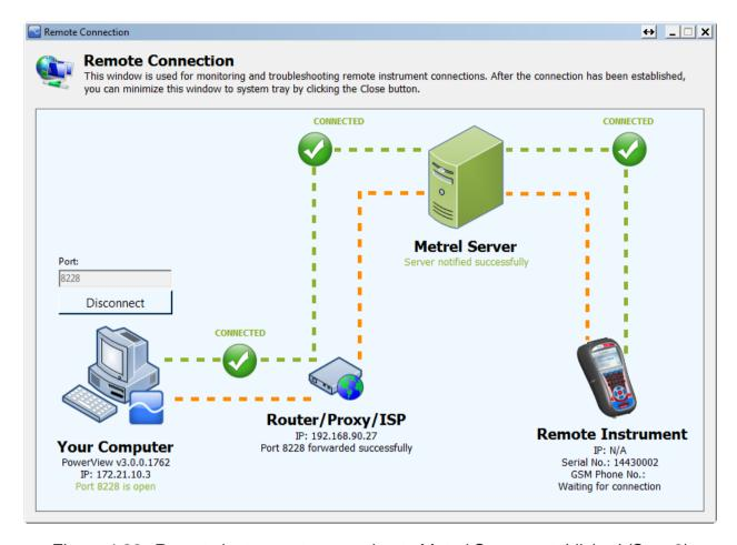
Figure 4.28: Remote instrument connection to Metrel Server established (Step 3)
