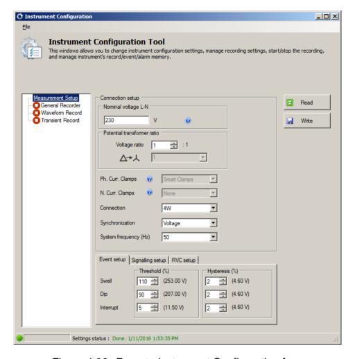
Figure 4.36: Remote Instrument Configuration form
