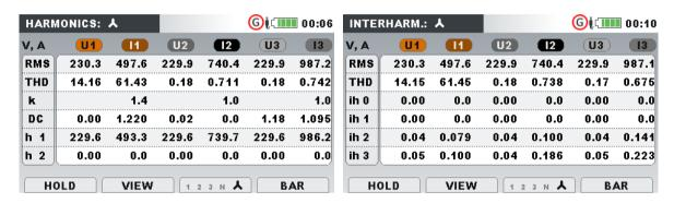
Figure 3.30: Harmonics and interharmonics (METER) screens
