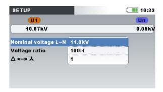
Figure 4.13: Voltage ratio for 11 kV / 110 kV transformer example
