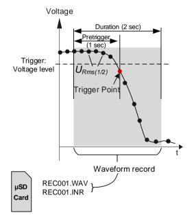
Figure 5.19: Voltage Level Triggering
