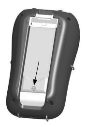
Figure 7.2: Closing the battery compartment cover
