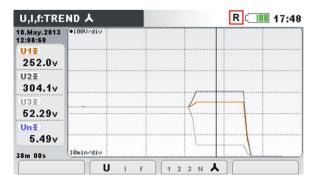
Figure 3.61: Viewing recorder U,I,f TREND data
