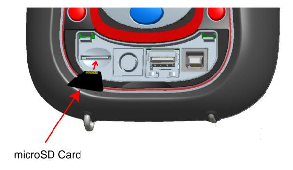
Figure 3.4: Inserting microSD card
