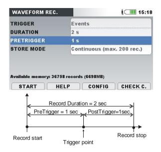
Figure 5.17: Triggering and pre-triggering description
