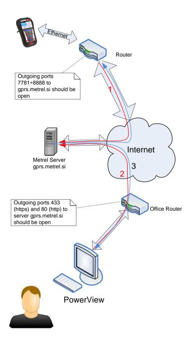
Figure 4.23: Schematic view on the remote measurements
