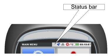
Figure 3.3: Instrument status bar
