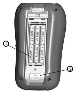
Figure 7.1: Battery compartment
