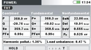
Figure 3.25: Detailed total power measurements
