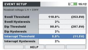
Figure 5.21: Waveform recorder setup for triggering on voltage events
