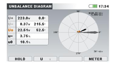
Figure 3.37: Unbalance diagram screen
