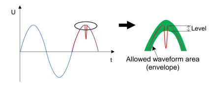
Figure 5.24: Transients trigger detection (envelope)
