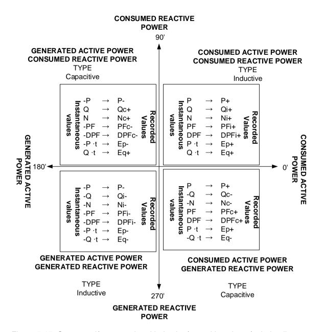
Figure 5.15: Consumed/generated and inductive/capacitive phase/polarity diagram
