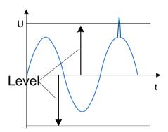
Figure 5.25: Transients trigger detection (envelope)
