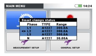
Figure 4.19: Automatically recognised clamps status
