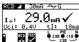
Figure 5.20: Example of trip-out current measurement result
