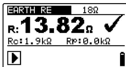
Figure 5.35: Example of earth resistance measurement result
