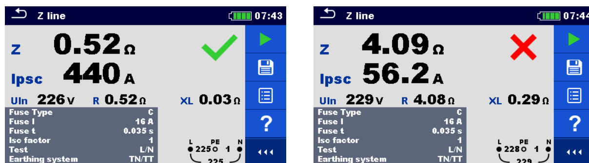
Figure 7.44: Examples of Line impedance measurement result
