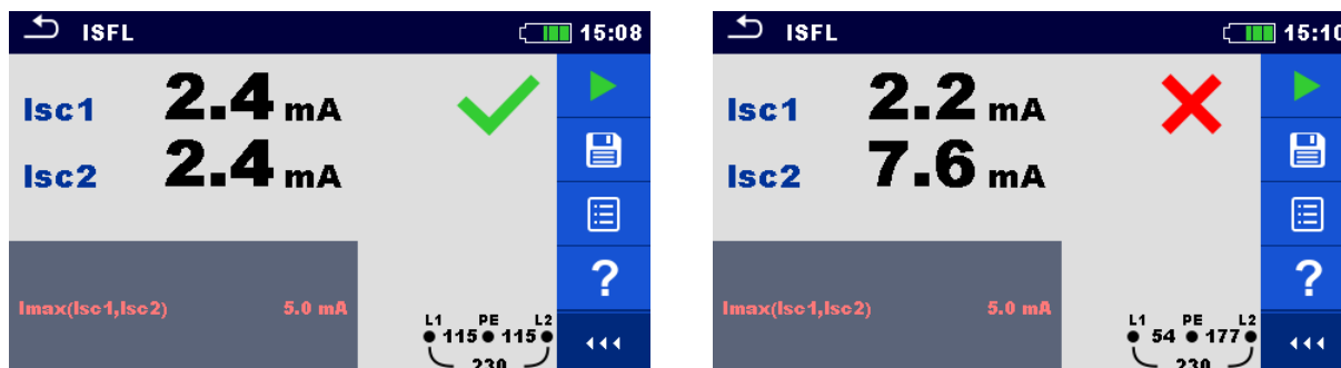
Figure 7.74: Examples of First fault leakage current measurement result
