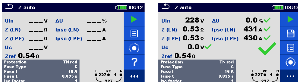
Figure 7.98: Example of Z auto measurement results
