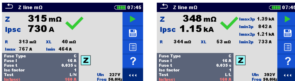
Figure 7.47: Examples of high precision Line impedance measurement result
