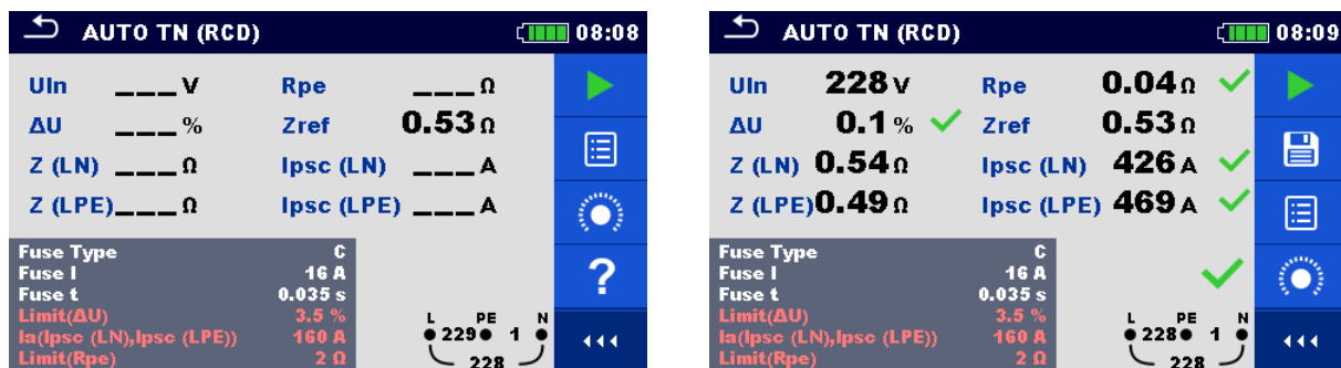
Figure 7.89: Examples of AUTO TN (RCD) measurement results
