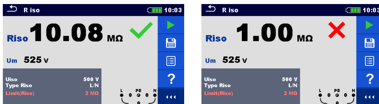
Figure 7.9: Examples of Insulation resistance measurement result
