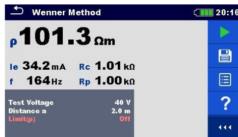
Figure 11.45: Example of Wenner method measurement result
