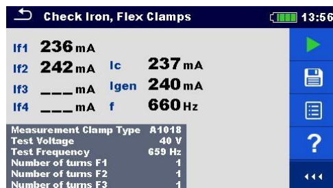
Figure 11.104: Example of Check Iron, Flex Clamps measurement result
