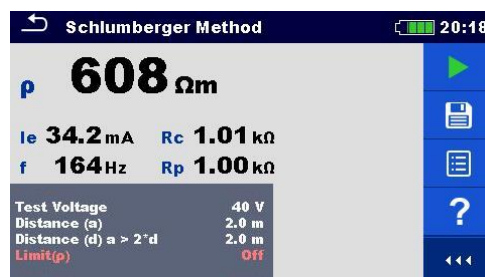
Figure 11.48: Example of Schlumberger method measurement result
