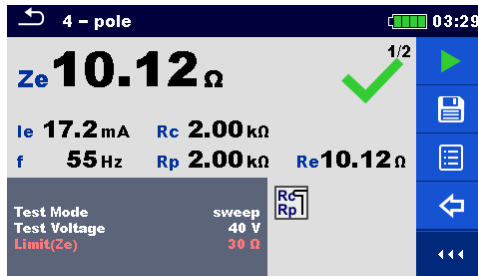
Figure 10.2: Single test result screen Example of 4 -pole measurement
