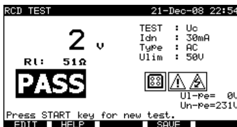
Example of contact voltage measurement results
