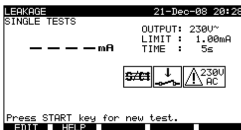
Differential leakage current menu
