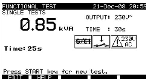
Example of apparent power measurement result
