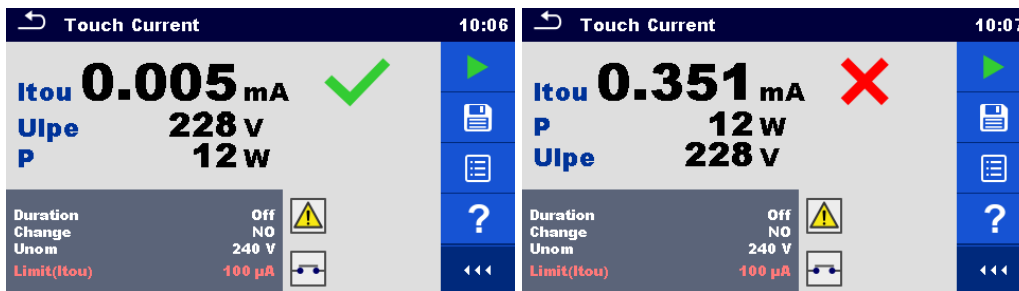
Figure 6.104: Examples of Touch current measurement results
