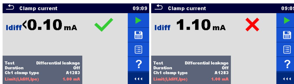
Figure 6.74: Examples of Clamp current measurement results
