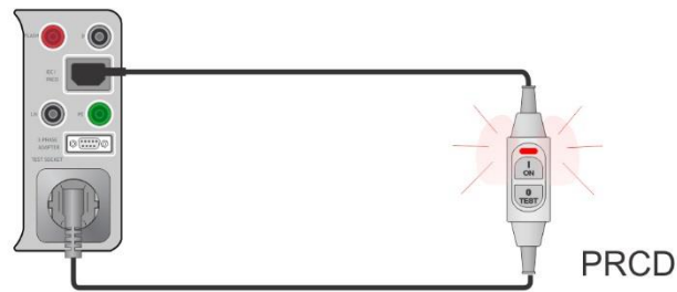
Figure 6.62: Open conductor (PRCD) test
