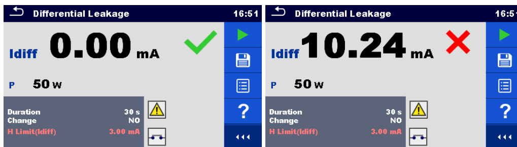
Figure 6.39: Examples of Differential Leakage measurement results
