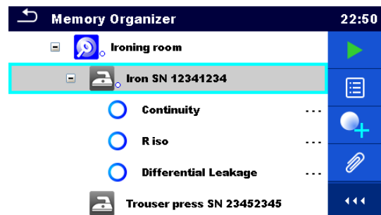
Figure 5.3: Example of status - No measurement result(s)
