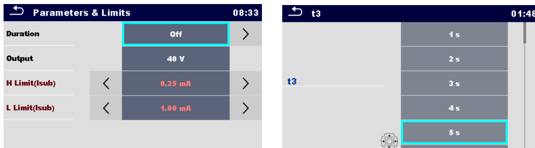
Figure 6.3: Screens in menu for setting Single test parameters and limits
