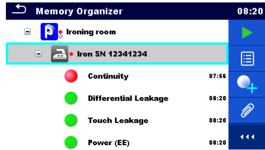
Figure 5.6: Status - Measurements completed with fail result(s)
