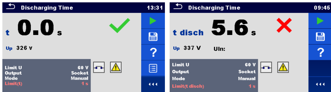
Figure 6.65: Examples of Discharging Time measurement results (Output = Socket)
