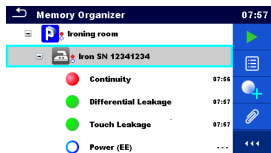
Figure 5.5: Example of status - Measurements not completed with fail result(s)
