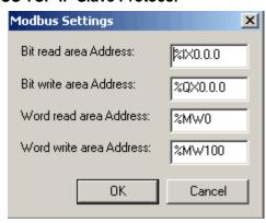
Instead of proprietary MLDP server protocol as above, the FEnet module can be configured to serve open standard MODBUS TCP-IP slave protocol for allowing any third-party controllers / HMI / SCADA to communicate with MasterLogic PLCs.
