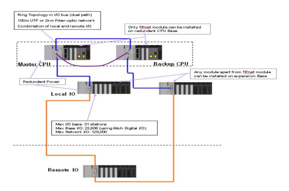
The above diagram demonstrates co-existence of both local I/O base and remote I/O base (i.e. UTP and fiber-optic cables) in a single I/O network.
