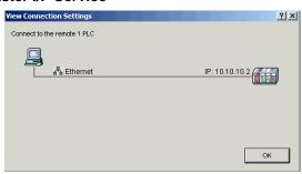
Every FEnet module has a ready built-in service for SoftMaster using TCP-IP Port 2002. This service is automatic and can be in the background along with other services.
