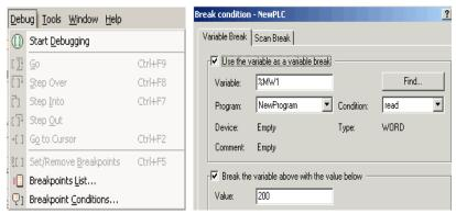
MasterLogic-200 program can be optionally started in DEBUG mode for any specific trouble-shooting. Breakpoints can be either:
