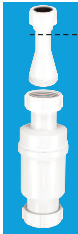
MacValve 1 1/4" BSP female inlet nut x 1 1/4" universal compression outlet including Tundish adaptor 1 1/4" BSP male thread x 22mm universal inlet
